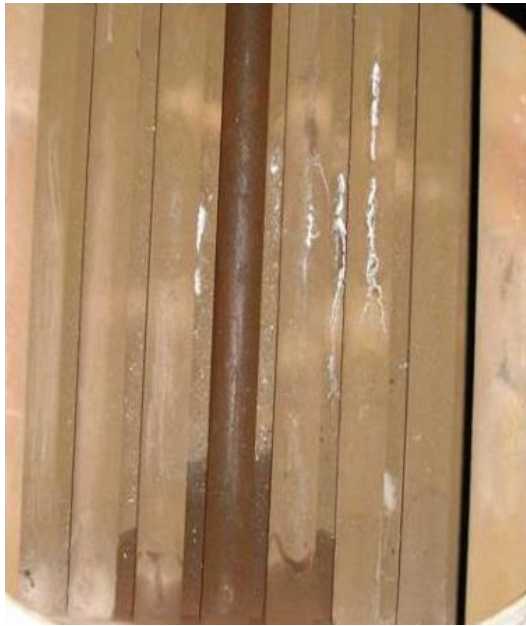
Scaled boiler tubes before cleaning boiler tubes after chemical clean
